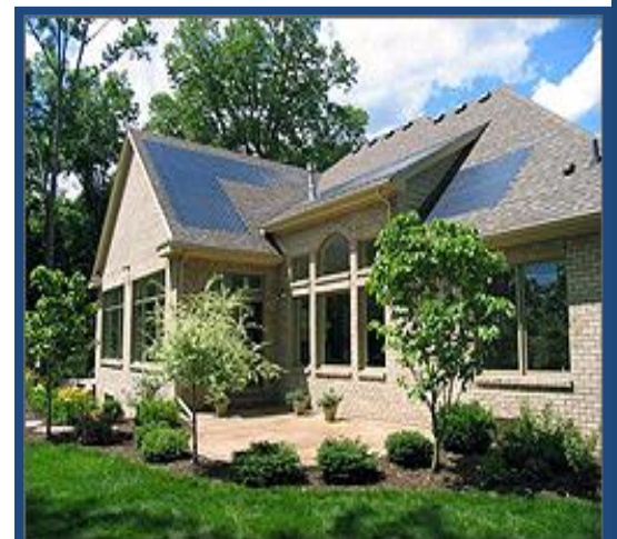
Solar PV roof shingles provide a unique alternative to traditional roof-mounted solar. Photo credit: NREL
